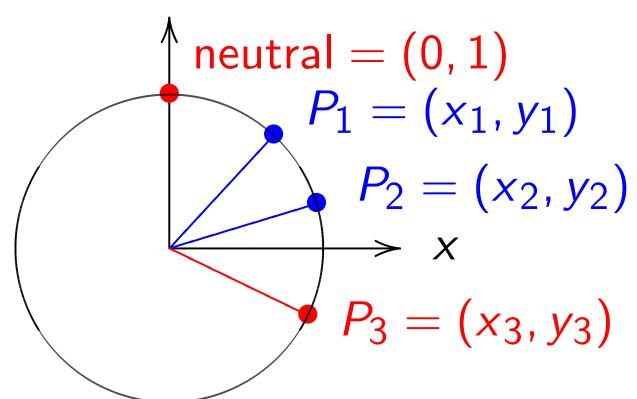
Use Cartesian coordinates for addition. Addition formula for the clock  $x^2 + y^2 = 1$ : sum  $(x_1, y_1) + (x_2, y_2) = (x_3, y_3)$  =  $(x_1y_2 + y_1x_2, y_1y_2 - x_1x_2)$ . Note  $(x_1, y_1) + (-x_1, y_1) = (0, 1)$ .  $kP = \underbrace{P + P + \cdots + P}_{k \text{ copies}}$  for  $k \ge 0$ .
