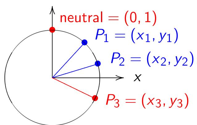
Use Cartesian coordinates for addition. Addition formula for the clock  $x^2 + y^2 = 1$ : sum  $(x_1, y_1) + (x_2, y_2) = (x_3, y_3)$  $=(x_1y_2+y_1x_2,y_1y_2-x_1x_2).$ Note  $(x_1, y_1) + (-x_1, y_1) = (0, 1)$ .  $kP = P + P + \cdots + P$  for  $k \ge 0$ . k copies
