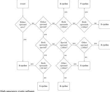
Flow chart for UMLAL (unsigned multiply add) from A performance study of X25519 on Cortex-M3 and M4 by Wouter de Groot.
